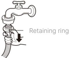
8. To install the water supply hose, please turn the retaining ring of the water supply hose back to release it.
