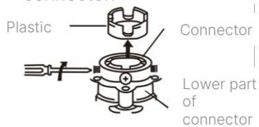
3. Adjust the four screws of the connector evenly so that two screws near the wall are fully in contact with the exterior of the faucet first.
