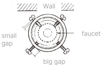
4. Hold the upper part of the connector against the mouth of the faucet so that the seal ring in the connector is fully in contact with the faucet (please do not take out the seal ring).
