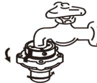
5. Rotate two screws (see figure below) opposite to the wall so that they are in contact with the faucet, and screw them with a screwdriver tightly.
