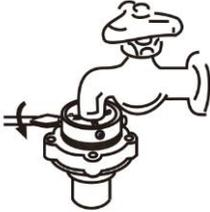
6. Rotate the lower part of the connector to screw it tightly (or else, water may leak from the connection). After rotation, the clearance between the lower part and the upper part of the connector shall be lower than 3mm.
